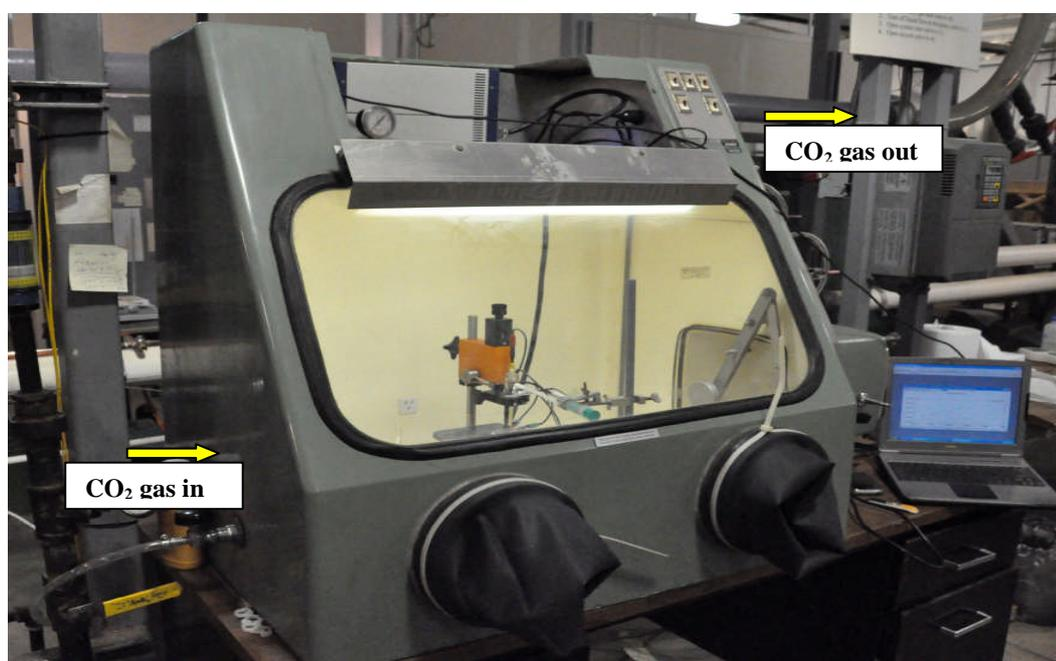
Figure 122. Micro electrochemical cell setup in a glove box.
